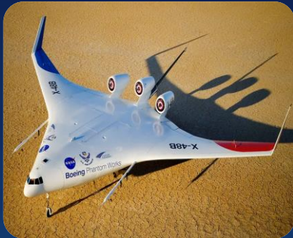
Designed & manufactured sub-scale blended wing flight test vehicle
